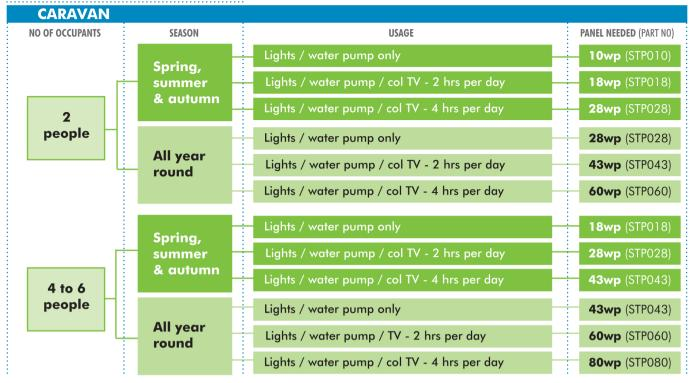
NOTE - If an additional hour's TV is needed or you use an inverter to power any devices, go up one panel size
