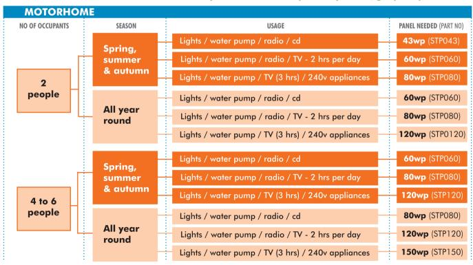
NOTE: if an additional hour's TV is needed, go up one panel size (for the last example above this means specifiying 2 panels – an STP080 and an STP120. Speak to your dealer about this.
